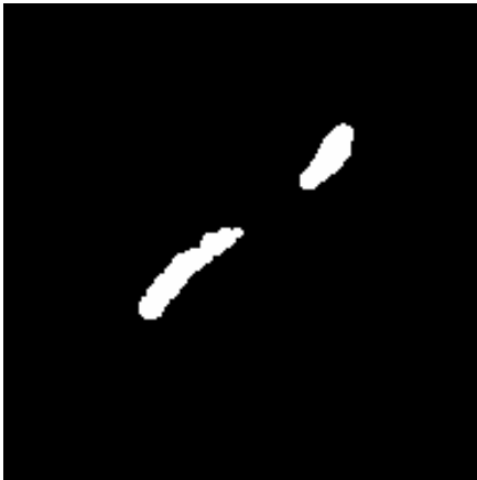
Fig. 10. A 2D slice of the “bit mask” produced by rasterizing the pearl string using the GPU-based implementation. White pixels indicate the voxels which are marked as “sent,” while black pixels indicate that the voxels are “unsent.” Note the ridges between adjacent voxels produced by this approach, which are not present in the final voxel extraction tool using the 2D region-growing implementation.
